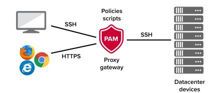
Imprivata Privileged Access Management addresses these challenges by controlling access time and locations, hiding privileged credentials from the end users, enforcing multifactor authentication, and approval workflow during access. The solution maintains password complexity and periodic update of credentials or SSH keys, ensuring least privilege principle by controlling what users can do on the servers and tracking privileged access to personal accounts or API tokens.
